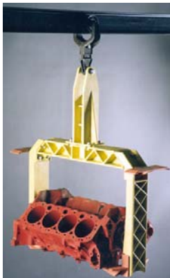
Plastic monorail carriers, such as the engine hanger shown above, offer many advantages over traditional alternatives
