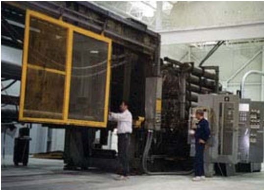
Molding large, custom returnable packaging and material handling products on one of Creative Techniques' structural foam machines.
